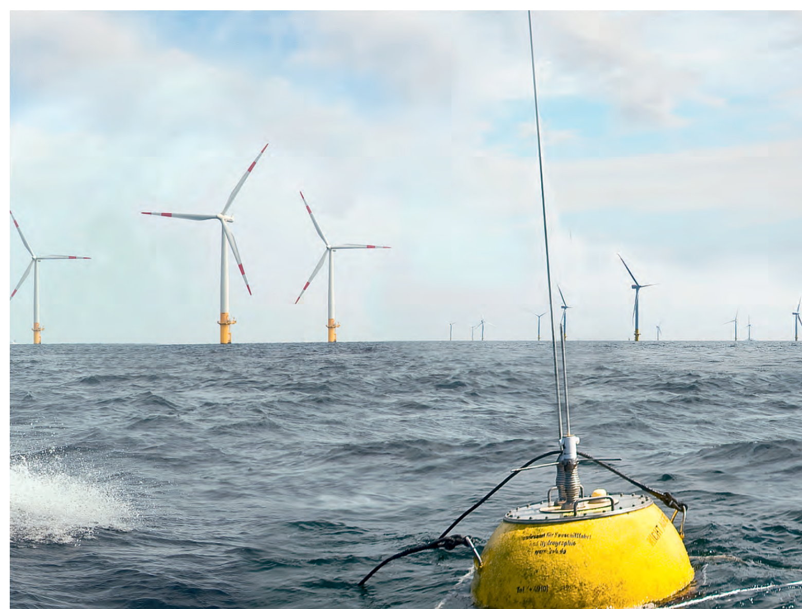
Fig. 1: Directional wave rider buoy at the wind farm Nordsee One.
